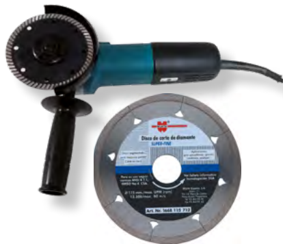
Radial tile saw + diamond blade cutting disc (Würht Super-Fine)
